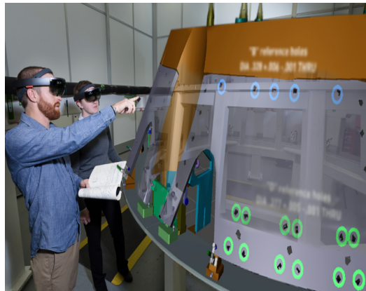
〈자료〉 MIT Technology Review, "NASA is using HoloLens AR headsets to build its new spacecraft faster", 2018. 10. 9.
